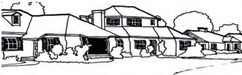
This house has both a varied front setback and the second story has been setback farther than the first floor wall.
