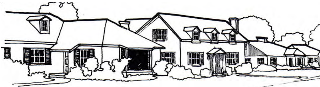
The mass of this house is reduced by lowering the plate height, using dormers and including an entry element.
