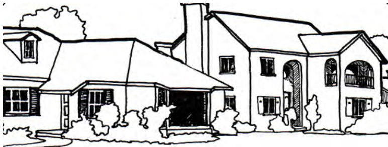
The house on the left has an entry with human scale, the one on the right does not.
